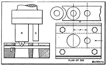
Fig. 2. Follow Die for Piercing and Blanking Washer
